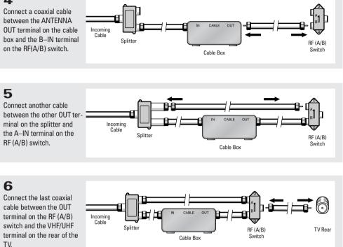
After you've made this connection, set the A/B switch to the "A" position for normal viewing. Set the A/B switch to the "B" position to view scrambled channels. (When you set the A/B switch to "B", you will need to tune your TV to the cable box's output channel, which is usually channel 3 or 4.)
