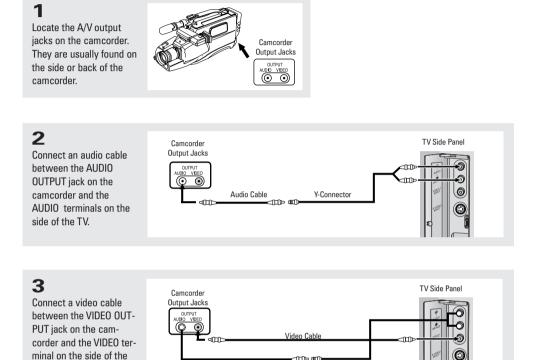
The audio-video cables shown here are usually included with a Camcorder. (If not, check your local electronics store.) If your camcorder is stereo, you need to connect a set of two cables.
