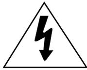
This symbol indicates high voltage is present inside. It is dangerous to make any kind of contact with any inside part of this product.
