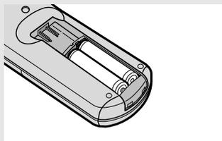
◀ Make sure to match the “+” and “-” ends of the batteries with the diagram inside the compartment.
