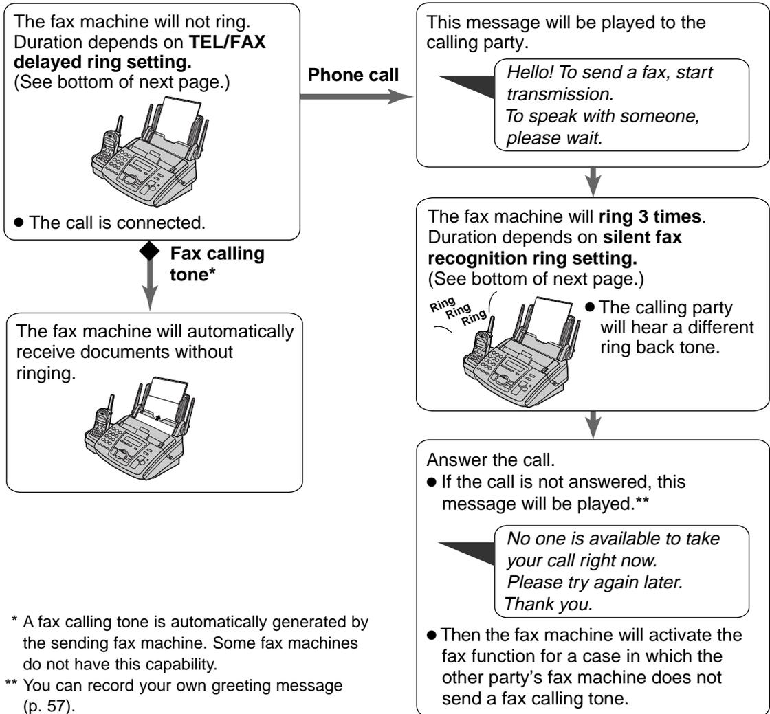
\* A fax calling tone is automatically generated by the sending fax machine. Some fax machines do not have this capability.
