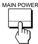
When the TV is turned on in the standby mode, the POWER indicator on the TV lights up. To turn on the TV completely, press POWER on the remote commander or the TV. When the TV is turned on completely, the PROGR +/-, VOLUME +/-, and TV/VIDEO indicators on the TV light up.
