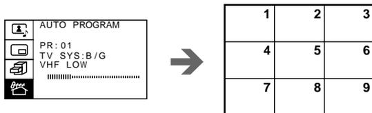
The TV starts scanning and presetting channels automatically. When all of the receivable channels are stored, the AUTO PROGRAM menu disappears and the first nine preset TV programs appear on the nine sub screens. The nine sub screens disappear after being displayed for several seconds.
