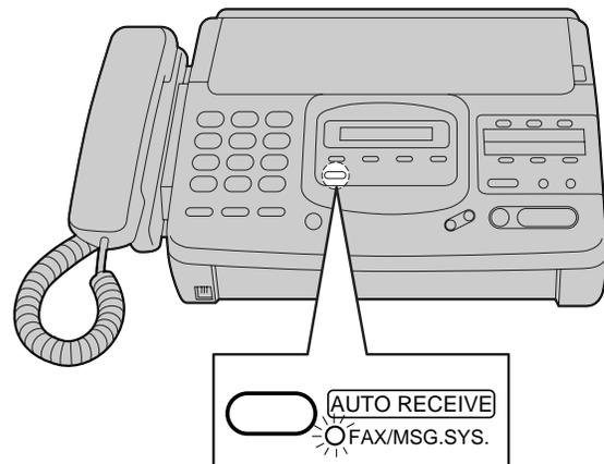
The FAX/MSG.SYS. indicator is on.
