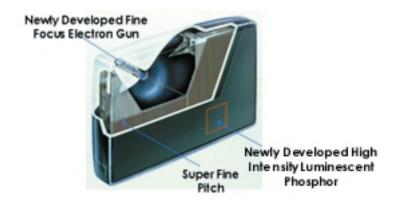
**SuperFine Pitch** provides better image detail with high definition sources. The Aperture Grill was improved by making the vertical slits a finer pitch that increases the number of slits by up to 65%(16 x 9 base). Also improved were the High Precision Deflection Yoke, Fine Focus Electron Gun and the inclusion of higher intensity Luminescent Phosphors. The result is a more detailed image for both moving and still images, higher resolution picture quality, and better edge detail.
