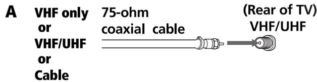
Use option A to connect the TV to a cable system or an antenna with a 75-ohm cable (usually built into newer homes).
