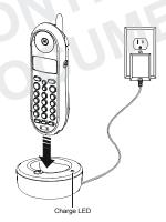
7 Charge the battery for at least 15 hours before using for the first time. The glowing LED light indicates that the handset is charging.
