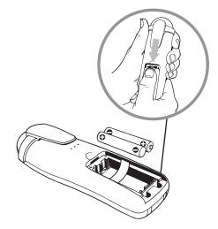
Insert the two batteries supplied, as indicated on the markings inside the battery compartment and slide the battery compartment shut. The handset display will show -!-. This means one handset is registered to the base. (If you have purchased the BT Freelance XD 100 Twin the additional handset will show -2-. See page 15.)
