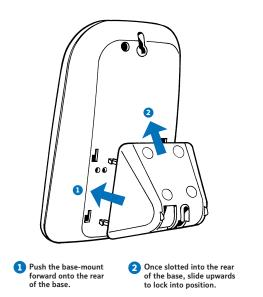
If wall mounting your BT On-Air 2100 SMS, use this guide for position.
