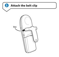
Fit the belt clip onto the back of the handset.
