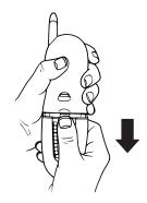
Unplug the connector and remove the old battery pack.
