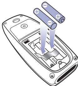
Replace the battery cover: hook the two plastic clips into place first, then lower and screw the cover into place. Finally, screw the belt clip on. You can use a coin, e.g. 10p piece if you don't have a screwdriver.
