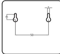
2. Insert the wall plugs provided into the holes and then insert the 2 screws, one into each hole. Leave a gap between the head of the screw and the wall (approx 3mm).
