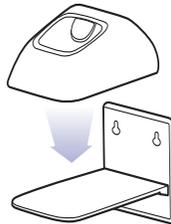
4. Fix the bracket (now with charger attached to it) onto the screws protruding from the wall, by placing it over the screw heads then pull it down gently and it should drop down and secure into place.
