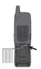
Plug the battery pack connector into handset.
