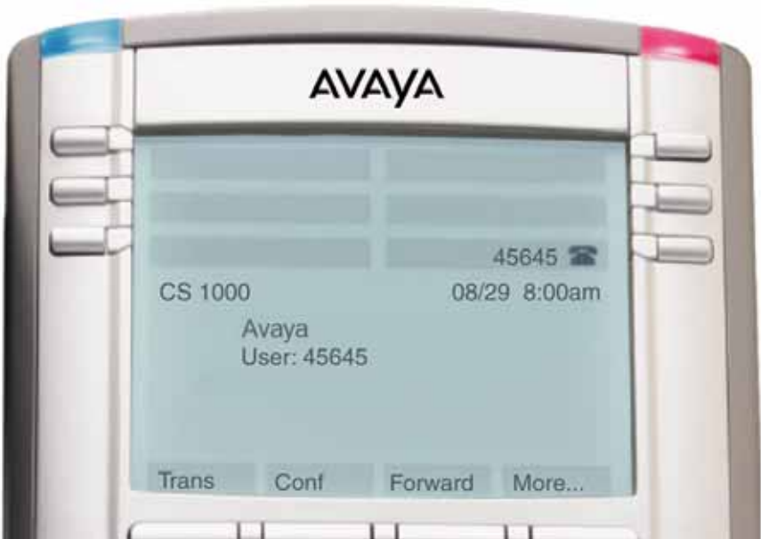
Figure 9: Logged in to an Avaya 1110 IP Deskphone using an Avaya 1140E IP Deskphone
