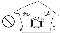
**8. Heat sources**---Do not install near any heat sources such as radiators, heat registers, stoves, or other apparatus (including amplifiers) that produce heat.
