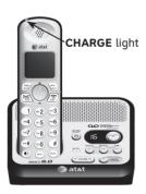
Charge the handset by placing it face up in the telephone base. The CHARGE light is on when charging.
