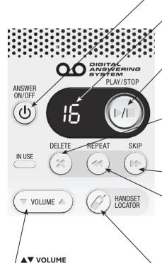
While the telephone is not in use, press to adjust the telephone base ringer volume (page 19).
