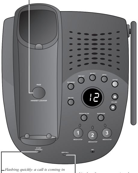
Flashing quickly: a call is coming inFlashing slowly: the handset is in useOn steadily: the handset is charging
