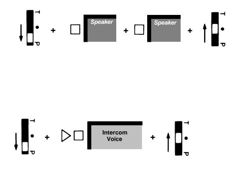
**NOTE:** If you plan to program other features when you program Automatic Line Selection, you must program Automatic Line Selection first. If you are already in the middle of a programming session, slide the T/P switch to center and then back to *P* before programming this feature.
