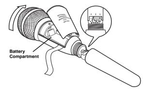
While holding the body of the microphone, carefully unscrew and remove the tapered lower section of the microphone.
