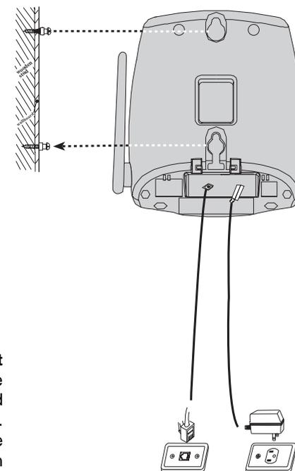
1. **Choose a spot near an electrical outlet and a telephone jack.** Your phone requires a modular telephone jack and a standard electrical outlet (120V AC). The power cord is six feet long; make sure there is an electrical outlet within reach of the base. The outlet should not be controlled by a wall switch. If the switch is ever turned off, the phone will not operate.
