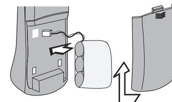
3. Plug the replacement battery cord into the Handset. Carefully snap the battery pack in place. Replace the battery cover by sliding it into place.
