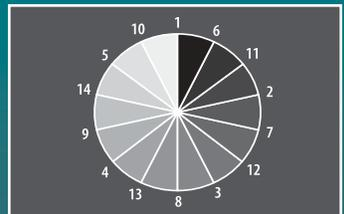
Synchronized RPM and BPM prevents overlapping impacts for 2X more efficient drilling
