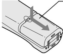
**2** Connect the battery pack connector with the correct polarity (black and red wires), then insert the battery pack into the battery compartment.
