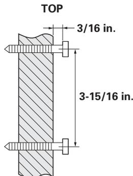
**1** Insert two mounting screws into the wall, (with their appropriate anchoring device), 3-15/16 inches apart. Allow about 3/16 of an inch between the wall and screwheads for mounting the phone.
