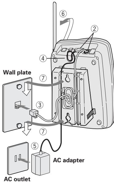
4 Wrap the AC adapter cord inside the molded wiring channel. Then wrap the cord around the strain relief notch.
