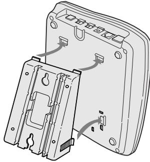
1 Snap the wall mount adapter into the notches on the base.
