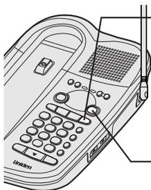
**1** During the conversation from the handset. Press and hold **voice memo** on the base. The unit begins recording and the LED blinks. A beep that can be heard by both parties sounds every 15 seconds.
