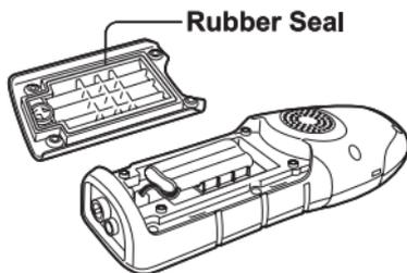
Note: If the rubber seal appears worn, nicked, or dried out, replacement seals are available through the Uniden Parts Department. See the back cover page for contact information.
