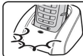
Make sure that the **charge LED** illuminates when the handset is seated.
