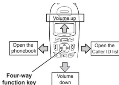
To use this four-way key, place your thumb over the key on the handset and move to the four positions to get the feel of how it moves and operates.
