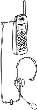
To connect the headset, open the rubber cover on the left side of the handset, then insert the headset's plug into the jack.
