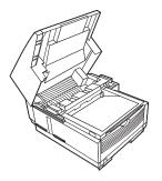
**3** Press the release buttons located on both sides of the copy stacker. Lift up the stacker.
