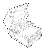
**3** Press on the latches on both sides of the copier stacker until the cover of the image drum compartment is released and pops up. Lift up and back, revealing the image drum.
