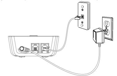
2. Plug one end of the telephone line cord in the LINE IN jack on the back of the base and the other end into a modular jack.
