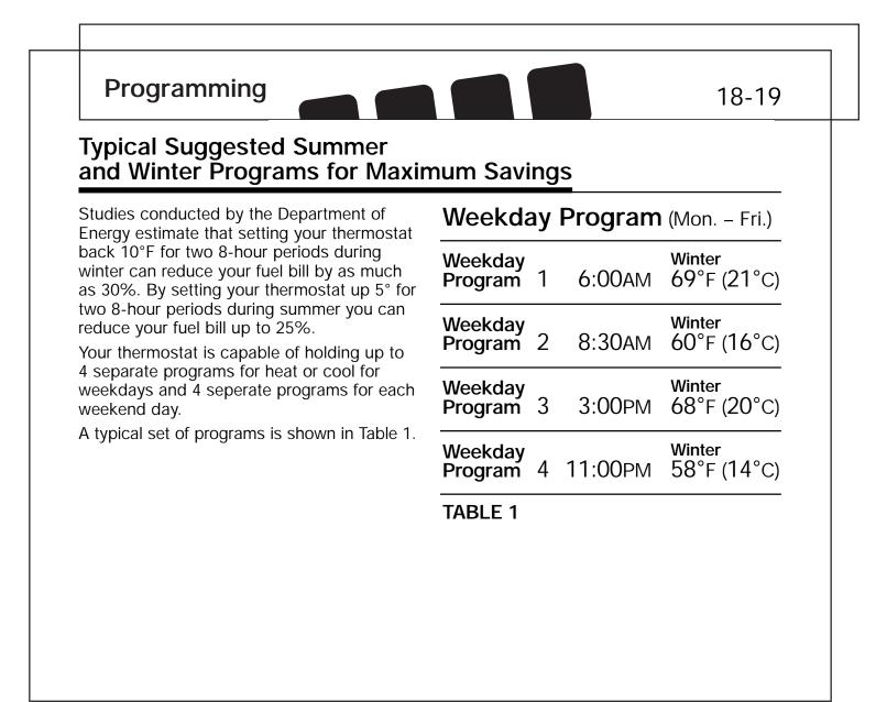
NOTE: The thermostat program will NOT take effect immediately after programming of your thermostat but at the next programmed time/temperature change. The thermostat is pre-set to 68°F (20°C) for heat and 78°F (25°C) for air conditioning. So if you want a temperature other than 68°F or 78°F (20°C or 25°C) right away, use the temporary manual override feature (described on page 26) to enter your desired temperature setting.
