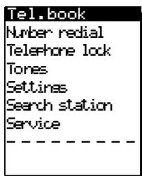
In order to select a function using the dialog key "OK," you must scroll with "NEXT" until the desired function is highlighted (dark background).
