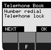
**The main menu is at** the left of the display. This appears after the F-key is pressed in idle status.
