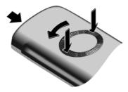
Insert a coin into the cavity at the top of the battery cover and twist it until the cover opens.
