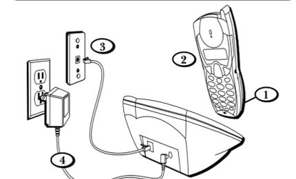
1. Remove the battery compartment door on the handset, insert the battery pack, plug the cord into the jack (inside the compartment), and replace the compartment door.
