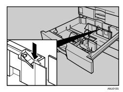
4 While pressing down the release lever, slide the side fences until they are aligned the paper size you want to load.
