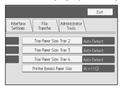
**5** Select the loaded paper size and feed direction, and then press [OK].
