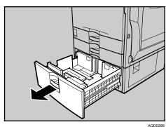
With the print side up, align all four sides of two paper stacks, and then load them next to each other in the tray. Each side has a limit of 1,000 sheets.
