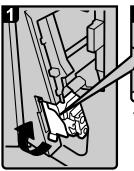
Open the front cover of the finisher, and then pull out staple unit.
