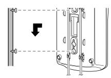
8. Press and lift out the handset holder, rotate it 180°, then snap it back into place so it holds the handset.
