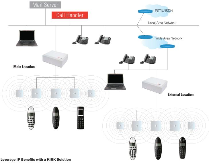
Above is an illustration of how the KIRK Wireless Server 1500 with IP interface is implemented in a business with two company locations, where the existing data network has been expanded to also include telephony. An IP-based call handler and a KIRK Wireless Server 1500 are installed at the main location, whereas the other is equipped with a KIRK Wireless Server 1500. Benefits of the solution include elimination of redundant
