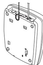
4. Route the adapter's cord through the strain relief slot on the base's bottom.
