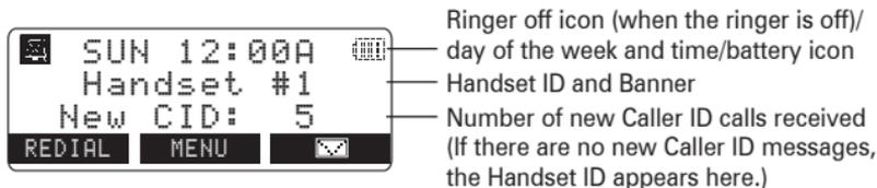
**NOTE** Illustration is of a single line system. Dual line systems will have different soft keys and standby screen.
