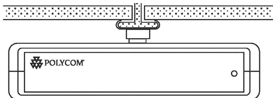
4. When properly attached the Base Station should sit almost flush against the ceiling and be tightly attached to the clip and T-bar grid work.
