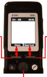
Right Softkey Pressing right softkey activates right softkey text.
