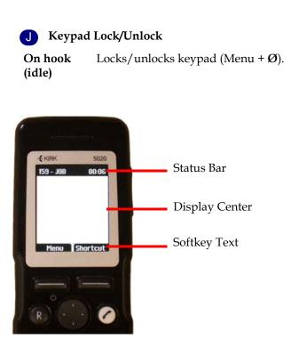
The display is divided in three parts: **Status bar**, **Display center** and **Softkey Text** (see figure above).
