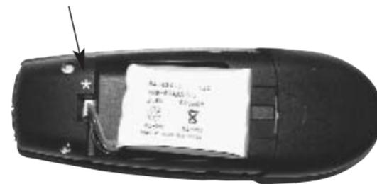
Place the battery plug in the slot with red wire closest to the mark \* (see figure)
