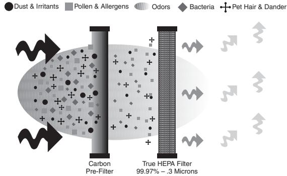
Fig. 1 - Illustration of the Air Filtration System
