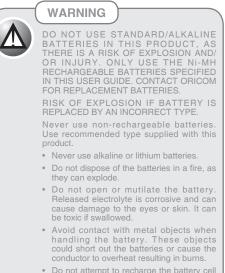
Do not attempt to recharge the battery cell by heating it. Sudden release of battery electrolyte can cause burns or irritation to the eyes or skin.
