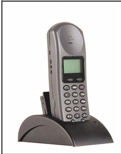
The Dual Charger is shipped with the appropriate power supply for the site. Place the Dual Charger on a flat, horizontal surface. Plug the power supply into the Dual Charger and into an appropriate wall outlet.
