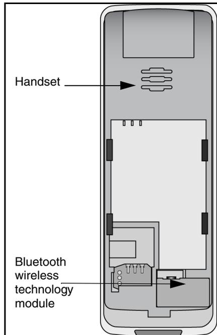
**Removing the Bluetooth wireless technology module from your DECT 4070 or 4075 Handset**
