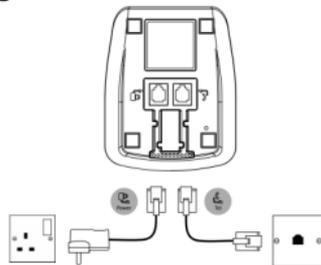
1. Plug the telephone line cord into the socket marked
