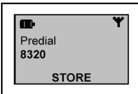
1. From Standby mode, use the keypad to dial the telephone number (up to 26 digits) to be stored.
