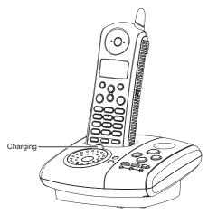
**Note:** Every time a battery is plugged in, the phone must be charged in the base for at least 10 seconds for the phone to properly restart.
