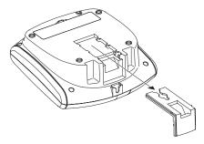
2 Turn the wall mount over so the key slot is facing upward. Align the holes of the wall mount with the feet of the base and push gently until the wall mount fits snugly into place.
