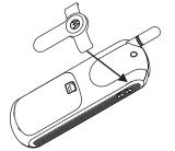
To remove the belt clip, gently release the tabs of the clip.
