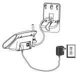
Insert the four tabs on the wall mount into the four slots on the back of the base then push down.
