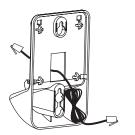
Plug the phone cord into the phone jack on the wall.Hang the bracket on the phone wall plate.
