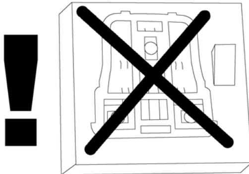
**NEVER** separately plug a plug-insert into a mains socket!
