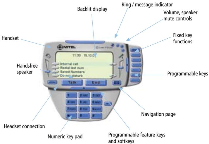
The Mitel 5110 Softphone is an IP extension on your PC / laptop. With the 5110 Softphone, users can log into their office extension from a remote location, allowing them to make and receive calls as though at their desk in the office. The Mitel 5110 Softphone is a component of the Mitel 3000 Communications System package that is available in 4, 8 or 12 user packages
