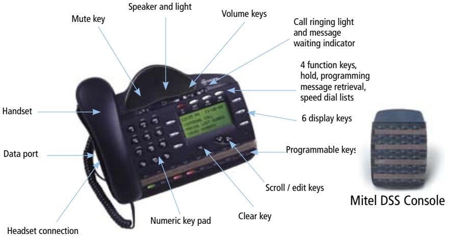
This Mitel 3000 digital feature phone includes a large easy to use display allowing the user to navigate the powerful features of the system. The Mitel DSS\* Console (direct station select) with 32 buttons can be added to the 4120 Telephone, making it a perfect solution for receptionists.
