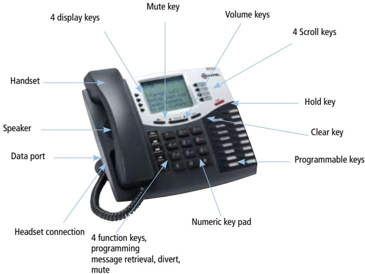
The Mitel 5120 IP Phone is what the remote worker has been waiting for! Whether working from home or a small branch office, the IP-based system phone offers flexibility without compromising functionality or professional image. In fact, the IP-based system phone can plug and play from anywhere in the office, home or branch office and all that is needed is a broadband connection.
