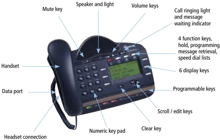
This Mitel 3000 digital feature phone includes a large, 4-line, easy-to-use display allowing the user to navigate the powerful features of the system. The programmable keys can be programmed as line keys (line 1, line 2, etc.), extensions (ext. 23, 24, etc.) or features (paging, forward, etc.)
